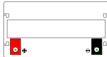
Battery bank spacing required 12.5mm (1/2"inch) minimum
