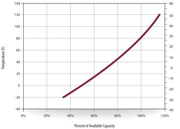
C.C.A. (Cold Cranking Amps) - the discharge load in amperes which a new, fully charged battery can maintain for 30 seconds at 0°F (-18°C) at a voltage above 1.2 V/cell.
